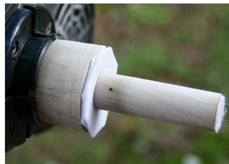
Slide the HF onto the shaft, turn away the chuck tenon, and shape the bottom of the vessel to leave a small nib that can be carefully sawed off and sanded flat. Voila. This simple jam chuck can be reused for other vessels with a similar mouth diameter. The length can be adjusted for shorter pieces by adding solid washers as shims at the top between the wood and the compressible washers.
