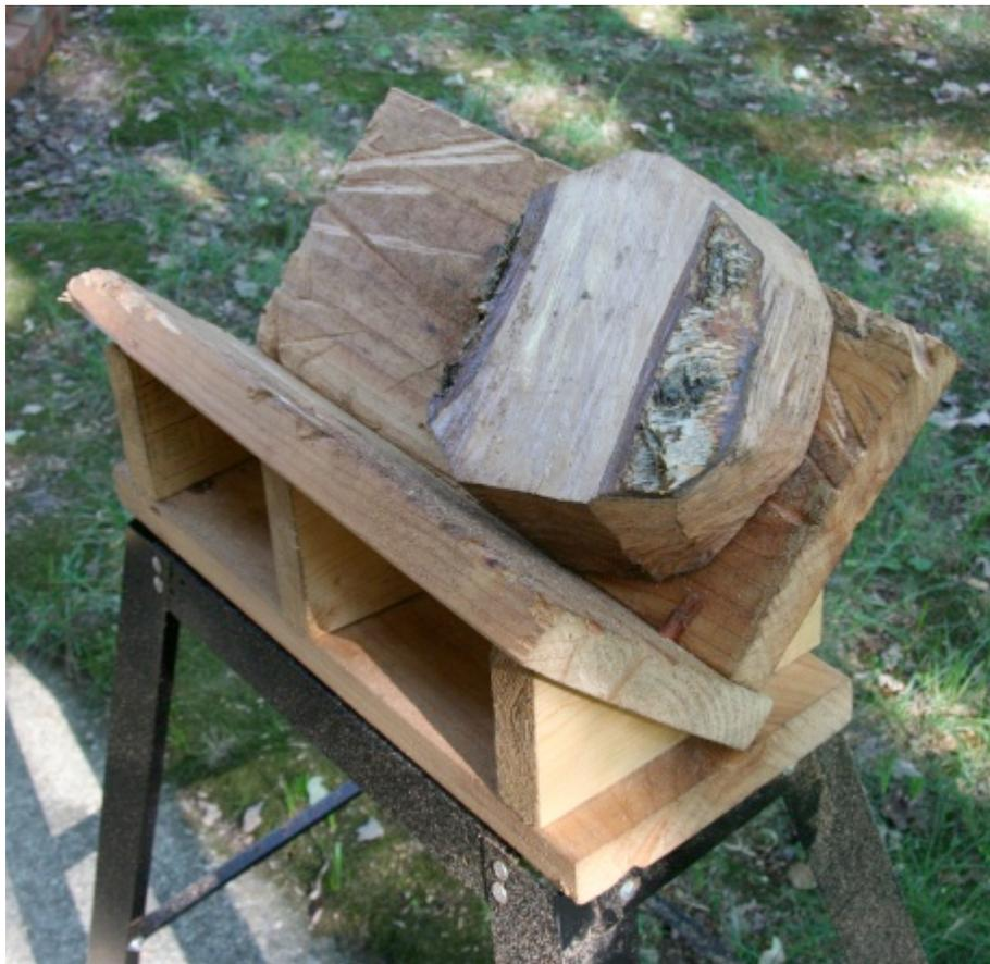
Because everything near the saw is wood, the chain can never come near metal – that’s important. There are obviously many improvements that could be made. The V boards can slide around a bit now, and might be pinned for further constraint, but I haven’t felt the need to make the effort. When I upgrade this one, I’ll use larger dowels for holding the top V board in place – a really heavy log could shear the small ones I used in mod 1.
