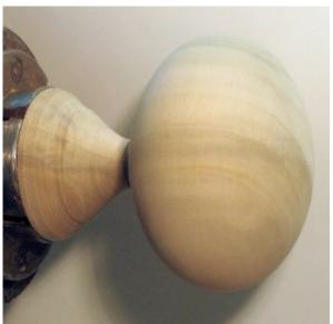
Note: This example was a test of the method for turning the outside shape. For a real ornament that will be hollowed, I recommend leaving more meat in the chuck-end connection for stability until after the hollowing is complete.
