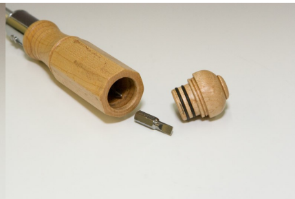
Mike Blake - hollow, octagonal screwdriver handle with O-rings
