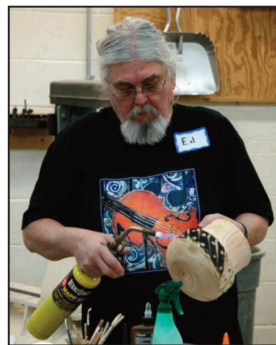
ED KARCH CHARRING A VESSEL WITH A MAPP TORCH
