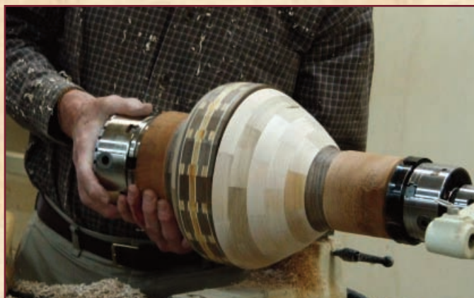
WITH THE OUTSIDE OF BOTH SECTIONS TURNED CLOSE TO FINAL SHAPE, FINAL TURNING, SANDING, & FINISHING ARE COMPLETED ON THE INSIDE. THE TAIL STOCK IS USED TO HELP ALIGN THE SECTIONS FOR GLUING AND HOLD THE SECTIONS TOGETHER WHILE THE GLUE DRIES.
