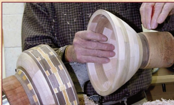
WITH THE GLUE SET, THE WASTE BLOCK IS PARTED OFF OF THE BOTTOM SECTION. FINAL SHAPING, SANDING, AND FINISHING IS COMPLETED. THE FINAL STEP IN THE PROCESS IS TO PART THE WASTE BLOCK OFF OF THE TOP SECTION AND CARRY OUT FINAL SANDING AND FINISHING. THIS PROCEDURE IS TOO COMPLICATED TO COVER HERE, BUT WILL BE ADDRESSED IN A FUTURE EDITION OF THE NEWSLETTER.
