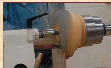
REVERSED WITH TENON IN CHUCK.
