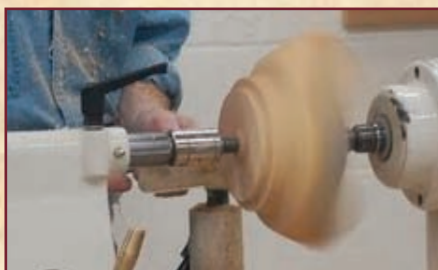
TENON FOR SCROLL CHUCK IS CUT.
