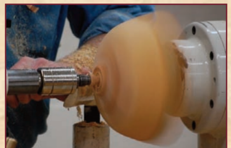
RECESS CUT IN FOOT & NIB REMOVED...
