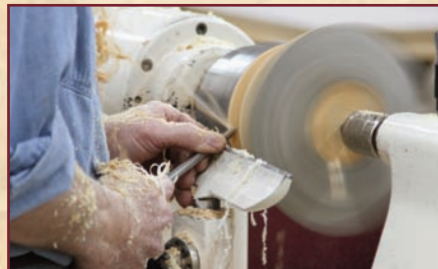
BACKWARDS SLICING CUT SHAPES FORM.
