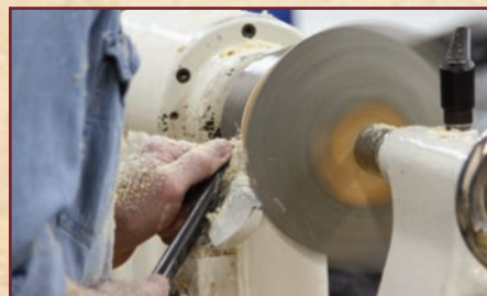
SHEER SCRAPING FINISHING CUT.
