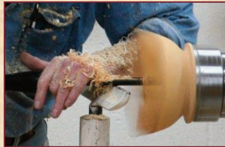
FINISHING CUTS TO COMPLETE INTERIOR ...TURN INSIDE TO MATCH OUTSIDE.
