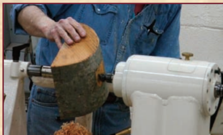
BLOCK MOUNTED BETWEEN CENTERS.
