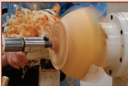
...IS CUT DOWN TO CREATE FOOT...
