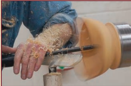
FINISHING CUTS TO COMPLETE INTERIOR ...TURN INSIDE TO MATCH OUTSIDE.
