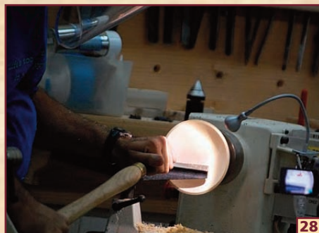
28 BACK TO THE BOWL, WITH A LIGHT DIRECTED TO THE SURFACE, WARREN TAKES VERY LIGHT CUTS TO REMOVE ANY TINY RIDGES REMAINING.
