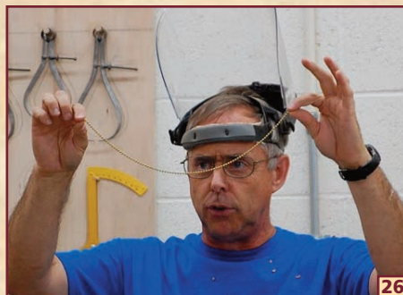
26 HE USES A LENGTH OF LAMP CHAIN, HELD AT BOTH ENDS, TO HELP DETERMINE THE INSIDE SHAPE OF HIS BOWLS, DEEP OR SHALLOW...
