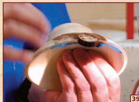
WARREN CAREFULLY BUILDS UP THE LEVEL OF DUST FILLER TO ENSURE ALL THE GAPS HAVE ENOUGH TO BOND WITH THE EDGES.
