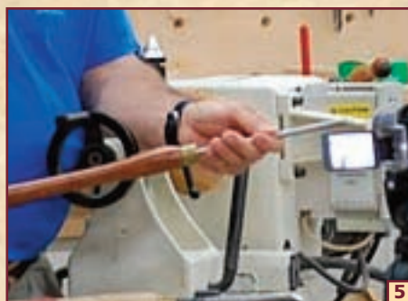
5 FOR FINE DETAILS AND SHAPING TENONS, WARREN USES A 1/4"-FLUTE GOUGE WITH A STANDARD BOWL GRIND.
