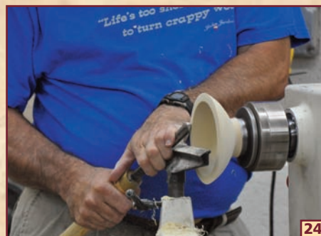
24 REVERSING THE BOWL AGAIN, HE USES THE INSIDE EDGE OF THE \frac{1}{2} " GOUGE AND LOWERS THE HANDLE TO SMOOTH THE RIM OF THE BOWL.
