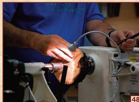
48 WARREN USES A PEN LIGHT BEAM TO TRACK OUTER SURFACE CUTS ON IRREGULAR SHAPED BURLS. HE CAN RE-POSITION THE PIECE TO AVOID PROBLEMS.
