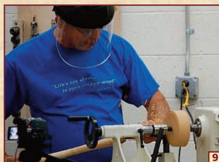
9 WITH A BETTER VIEW, YOU CAN SEE THE BLANK IS MOUNTED WITH A MORSE-TAPER DRIVE CENTER DIRECTLY INTO THE HEADSTOCK AND A REVOLVING... ↓
