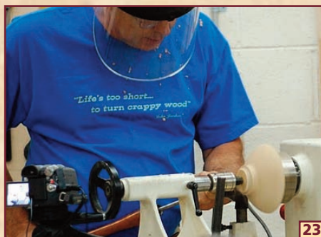
23 FIRST, HE USES THE STRONGHOLD CHUCK AS A "JAM" CHUCK, BRINGS THE TAIL STOCK BACK UP. AND WITH HIS \frac{1}{4} " GOUGE, REFINES THE CURVE OF THE FOOT.
