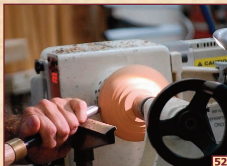
52 SINCE BURLS MOST OFTEN DO NOT HAVE A GRAIN "DIRECTION" LIKE SIDE- AND END-GRAIN PIECES, YOU DO NOT HAVE TO WORRY ABOUT CUTTING...
