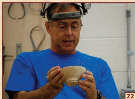
22 WARREN REMOVES THE BOWL AND CAREFULLY CHECKS BOTH SURFACES FOR ANY IRREGULARITIES THAT WOULD BETTER BE REMOVED WITH A GOUGE.
