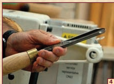
4 THIS 1/2"-FLUTE GOUGE WITH DAVID ELLSWORTH'S SWEEP BACK GRIND IS THE TOOL WARREN USES FOR ABOUT 90% OF HIS TURNING.
