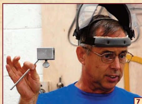
7 AND AN ELLSWORTH JIG TO MAINTAIN A CONSISTENT EDGE ON THE ELLSWORTH-GRIND GOUGES.
