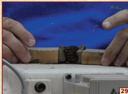
29 THIS "PATENTED" DEVICE... TWO SMALL BLOCKS WITH CURVED FOAM RUBBER PIECES ON EACH END HOLD THE WALNUT...
