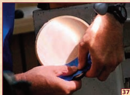
WHEN SATISFIED WITH THE FIT, WARREN APPLIES TAPE TO THE INSIDE TO HOLD THE SLICE IN PLACE AND TO KEEP THE GLUE FROM RUNNING.
