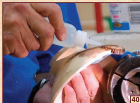
WITH A SMALL BOTTLE OF THIN CA GLUE AND A TINY OPENING, WARREN PUTS DROPS OF GLUE AROUND THE EDGES, QUICKLY BUT CAREFULLY.
