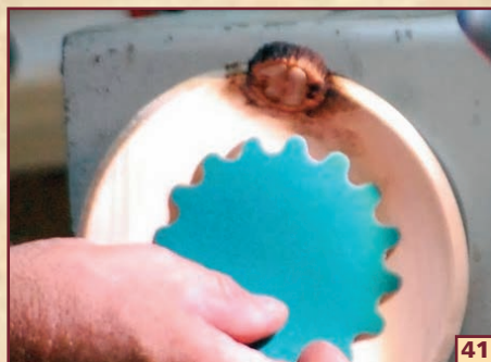
SANDING THE INSIDE OF THE SLICE FLUSH IS NEXT. WARREN LIKES WAVY-EDGE SANDING DISKS FOR THE INSIDE SURFACE, GOING FROM 80-GRIT TO 400-GRIT.
