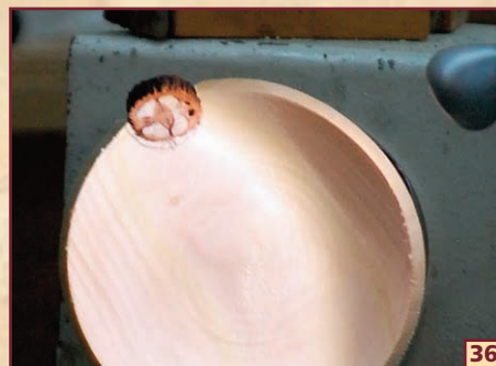
WARREN POSITIONS THE WALNUT IN THE GAP AND CHECKS FOR FIT. IT DOES NOT HAVE TO BE PERFECT, BUT BIG GAPS WILL CAUSE PROBLEMS.
