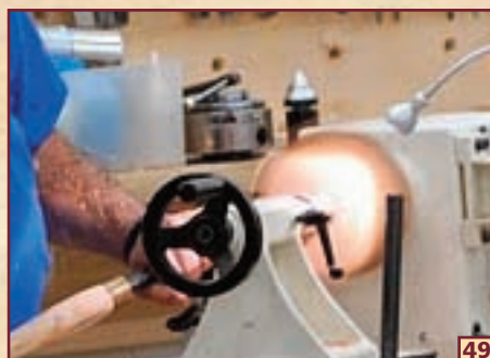
49 WITH THE AXIS CLEAR IN HIS MIND, WARREN BEGINS TURNING THE OUTSIDE TO CREATE THE BULB SHAPE HE WANTS FOR THIS PIECE.
