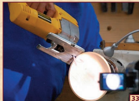
33 USING THE LATHE AS A VISE, WARREN ATTACKS THE UNSUSPECTING RIM WITH A JIG SAW...
