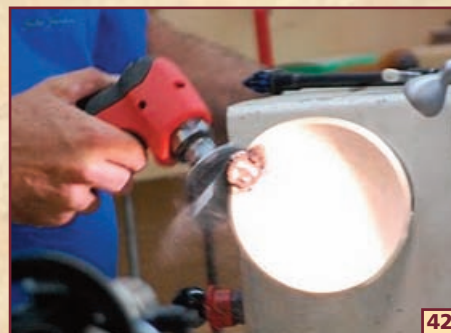
NEXT, WARREN SANDS THE OUTSIDE SURFACE TO REMOVE THE GLUE/DUST BUILD UP. THIS IS AS FAR AS HE TOOK THIS PIECE, SINCE TIME WAS LIMITED.
