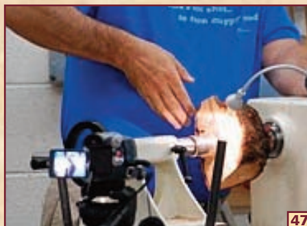
47 MOUNTING THIS PRE-CUT PIECE OF CHERRY BURL WITH A 4-PRONG DRIVE CENTER AND LIVE TAIL CENTER WITH THE POINT REMOVED.
