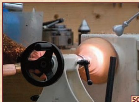
50 HE DEFINES THE TENON AND THE FOOT FIRST BECAUSE HE WILL USE THOSE TWO SECTIONS TO CUT TO AS HE CREATES THE SHAPE.
