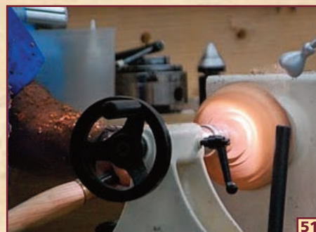
51 AS BEFORE, HIS FIRST FEW SHAPING CUTS MOVE OUT FROM THE TENON/FOOT TOWARDS THE RIM.
