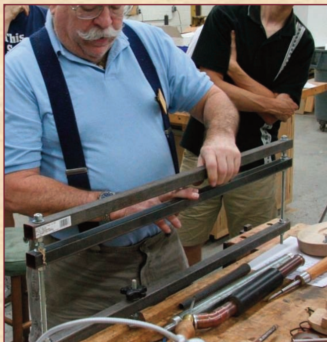
ELLIOT SCHANTZ BROUGHT SEVERAL INTRIGUING SHOP-MADE TOOLS, BUT THE MOST AMBITIOUS AND IMPRESSIVE WAS THIS LARGE REAR HOLLOWING BAR STABILIZER, PATTERNED AFTER THE LYLE JAMIESON MODEL. ELLIOT AND A FRIEND MADE THIS TOOL AT THE LEISURE WORLD WOODWORKING SHOP.
