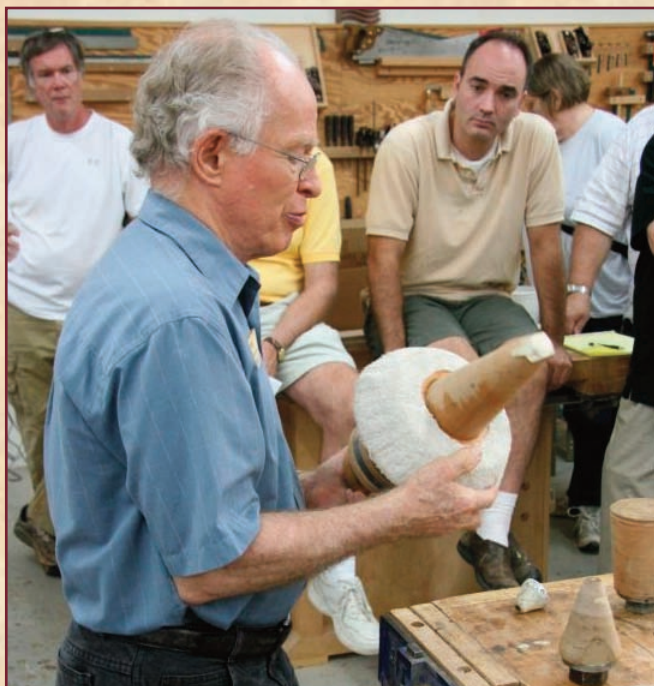
PHIL BROWN SHOWS A CONE-SHAPED CHUCK FOR HOLDING A DEEP VESSEL, WITH NO PRESSURE ON THE RIM, WHILE REMOVING THE SHOULDER AND CHUCK MARKS AND TOUCHING UP THE BOTTOM-RESTING SURFACE. THE PADDED CENTERING RING HOLDS THE RIM IN PLACE. TALL VESSELS WITH NARROW BASES MAY ALSO NEED AN INTERNAL SUPPORT.
