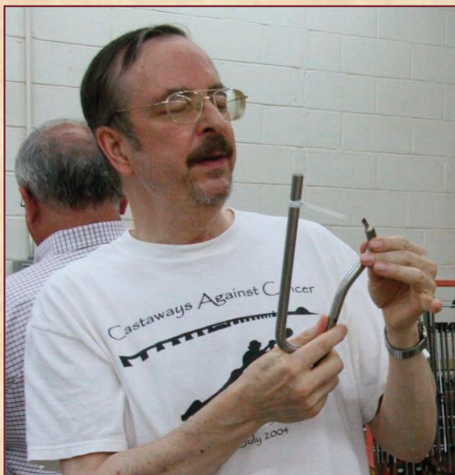
GARY GUENTHER BROUGHT A BENT HOLLOWING TOOL MOUNTED WITH AN "OUTRIGGER" OR "TORQUE ARRESTOR". THIS ONE WAS MADE BY C.A. SAVOY. THIS IS AN INEXPENSIVE, BUT VERY SECURE, METHOD FOR STABLE, COMFORTABLE, AND SAFE BLIND HOLLOWING.
