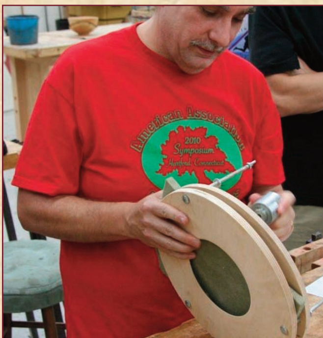
TIM ALEY BROUGHT A LARGE "MODULAR FACEPLATE SYSTEM" [OFTEN CALLED A DONUT CHUCK] MADE BY HIS FATHER-IN-LAW, MCW MEMBER DON COUCHMAN, TO FINISH THE BOTTOMS OF BOWLS, WITHOUT IMPEDIMENT.
