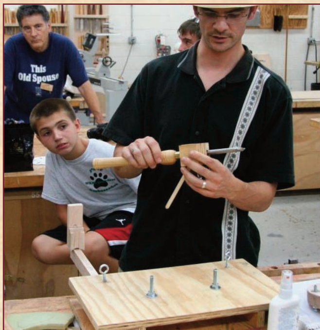
NEW MEMBER STEVE DiBENEDETTO MADE HIS OWN JIG OUT OF PLYWOOD TO MIMIC A WOLVERINE SYSTEM AND BROUGHT IT IN, MINUS THE GRINDER. THE 2 NUTS & BOLTS IN THE MIDDLE ARE WHAT HOLD THE GRINDER IN PLACE.
