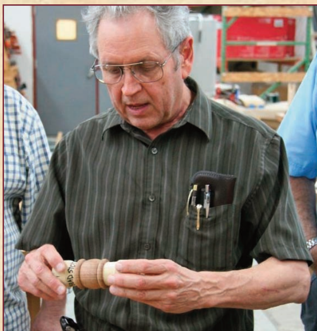
BILL AUTRY WAS RECENTLY HAD TO MAKE 24 MATCHING NAPKIN RINGS. AFTER TURNING A SPINDLE AND PARTING IT INTO SECTIONS, THIS IS THE JIG HE DESIGNED TO TURN THE RINGS, ACCURATELY AND QUICKLY, WITHOUT A CHUCK.
