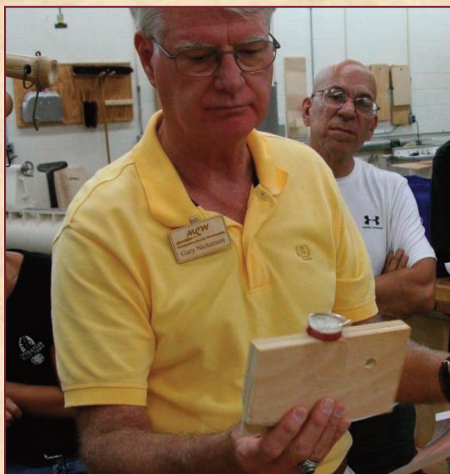
GARY NICKERSON MADE A LEVELED JIG FOR USE WITH AN ELLSWORTH SHARPENING JIG AND THE ELLSWORTH SIGNATURE BOWL GOUGE. THE JIG MAKES IT EASY TO SET HIS GRINDING WHEEL 7" FROM THE NOTCH AND 4" HIGH. HE ALSO BROUGHT A PHOTOGRAPH OF HIS GRINDER SET UP TO SHOW HOW THE JIG WORKS.
