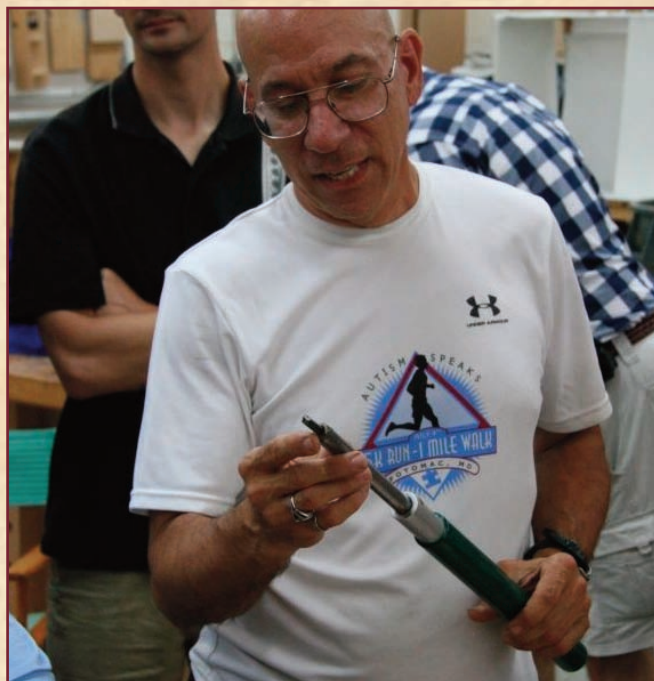
MICHAEL COLELLA SHOWED A ROUGHING TOOL, MADE FROM 5/8" BAR WITH 1/4" TOOL STEEL BIT IN A TRENT BOSCH-SIGNATURE ALUMINUM HANDLE.
