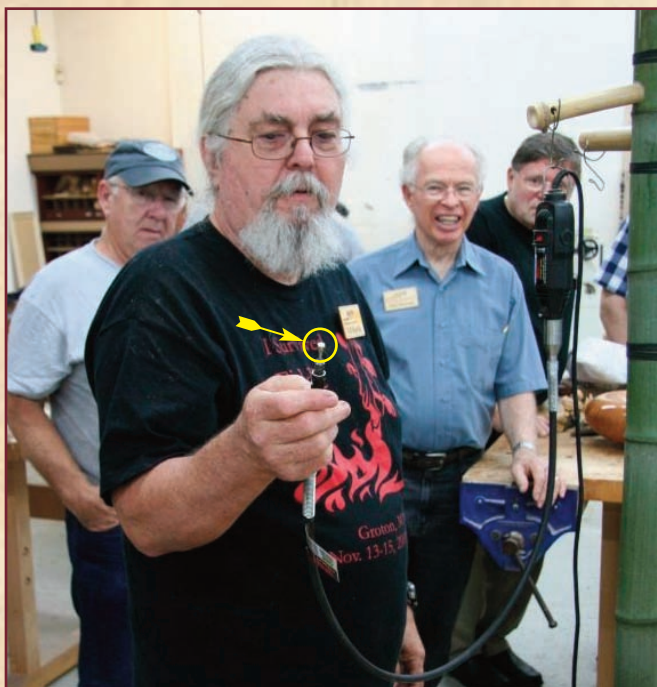
EVER INVENTIVE, ED KARCH BROUGHT HIS STAND FOR HOLDING FLEXIBLE CORD TOOLS LIKE THIS DREMEL. IN THIS SHOT A BAMBOO SHAFT PORTION OF THE STAND IS SEEN AT THE RIGHT... WHAT IS NOT VISIBLE IS A LEG/WHEEL SECTION OF A DESK CHAIR INSERTED IN THE END OF THE BAMBOO POLE. IN THE TOOL, IS CUTOFF WHEEL SHAFT WITH THE SCREW REMOVED SO HE CAN AFFIX TINY PIECES OF SANDPAPER FOR GETTING INTO VERY SMALL PLACES.
