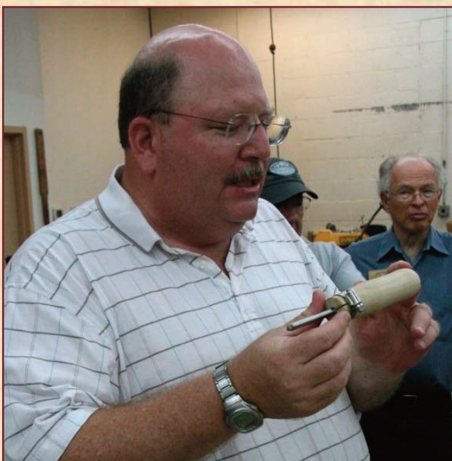
CARL POWELL BROUGHT A \frac{5}{16} " TRI-POINT TOOL IN A HANDLE(?) MADE LIKE A COLLET CHUCK, WITH A HOSE CLAMP. HE ALSO SHOWED TWO \frac{5}{16} " NUTS, DRILLED TO ACCEPT A \frac{5}{16} " BIT AND TAPPED FOR SET SCREWS TO HOLD IT IN PLACE TO GRIND THE ANGLES OF THE TRI-POINT TOOL PRECISELY 120° APART. [EDITORIAL COMMENTARY – APPARENTLY CARL SPENT SO MUCH TIME MAKING THIS STRANGE CONTRAPTION HE DID NOT HAVE TIME TO MAKE A REAL HANDLE.]
