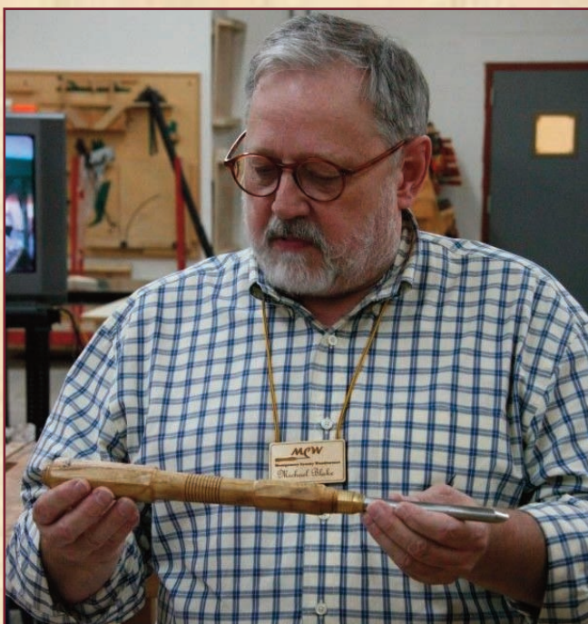
MICHAEL BLAKE BROUGHT THIS WOODCUT SPINDLE GOUGE. THE BLADE IS MADE IN NEW ZEALAND AND HAS A SOLID SHAFT, BUT THE FINAL 2" ARE A REPLACEABLE CUTTING TIP. THE TOOL IS VERY STABLE AND CAME WITH A "SCARY-SHARP" CUTTING EDGE. THE CUTTING EDGE IS ALSO RADICALLY SWEPT-BACK, SO IT CUTS SMOOTHLY WITH LITTLE EFFORT. THE JERRY GLASER-INSPIRED OCTAGON HANDLE WAS MADE FROM LIGHTLY SPALTED WHITE OAK.
