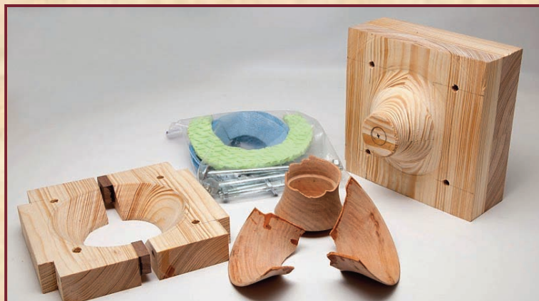
SHOP-MADE CHUCK SYSTEM FOR HOLLOWING FROM BOTH ENDS. BILL THINKS THE PIECE BLEW UP BECAUSE HE TRIED TO TURN IT TOO THIN.
