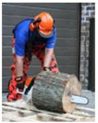
way through the log, and that the log should be turned 180° with the cut finished from the opposite side. The result will be two halves that are now ready to be trimmed and put on the lathe for turning.
