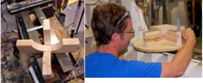
ing a masking tape interface between the workpiece and the holding jig pieces. Before the glue set, the workpiece was precisely leveled in relationship to the faceplate plane. The entire assembly was then mounted on the lathe and centered for the final turning, which comprises the
