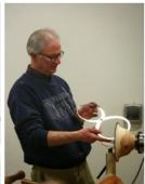
After the hollowing was completed and sanded, Mark re-mounted the bowl on a fitted jam-chuck for finishing the base or foot of the bowl.
