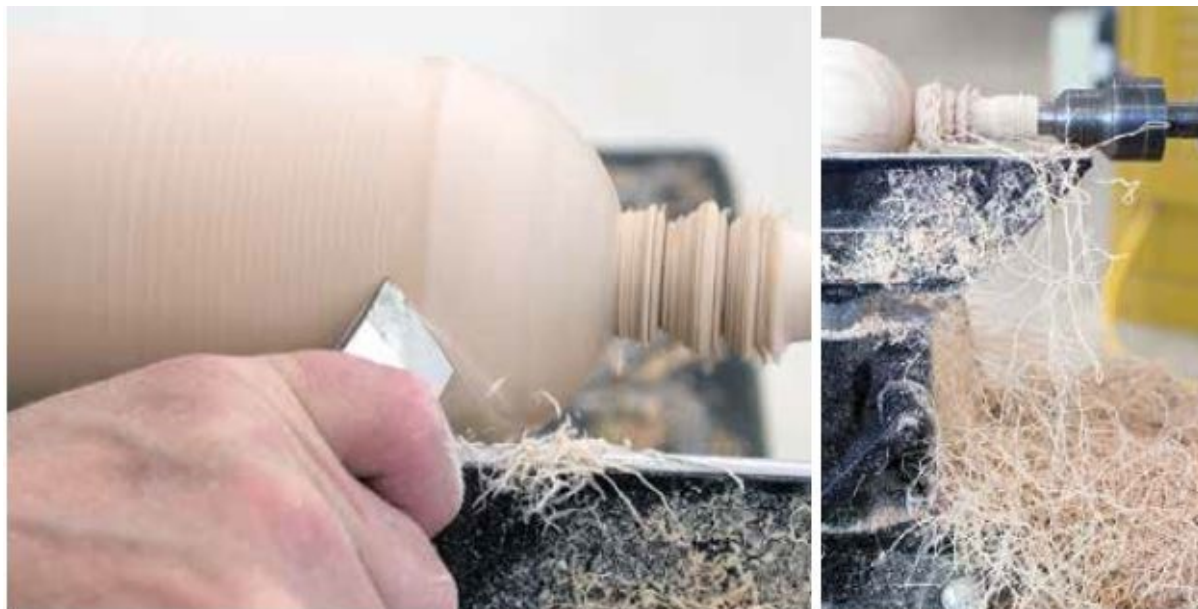
The fine “angel hair” shavings from a skew’s shearing cut indicate a clean cut along the wood’s sidegrain.
