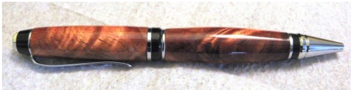
Matt made this large "cigar" pen in very curly koa, using a skew chisel to get a fine cut through the tricky, confused grain patterns. No sanding! CA glue finish. Nice job.
