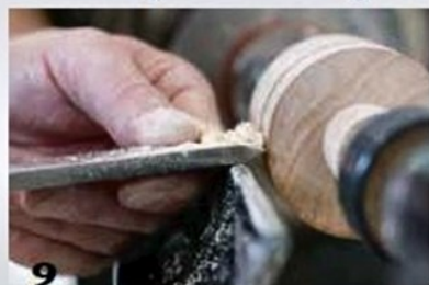
Three skew cuts, from left: scraping, peeling, and shearing. Each has its own angle of tool presentation and resulting pathway of shavings. The smoothest surface will result from the shearing cut, but each has its purpose.
