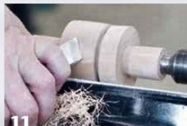
Three skew cuts, from left: scraping, peeling, and shearing. Each has its own angle of tool presentation and resulting pathway of shavings. The smoothest surface will result from the shearing cut, but each has its purpose.
