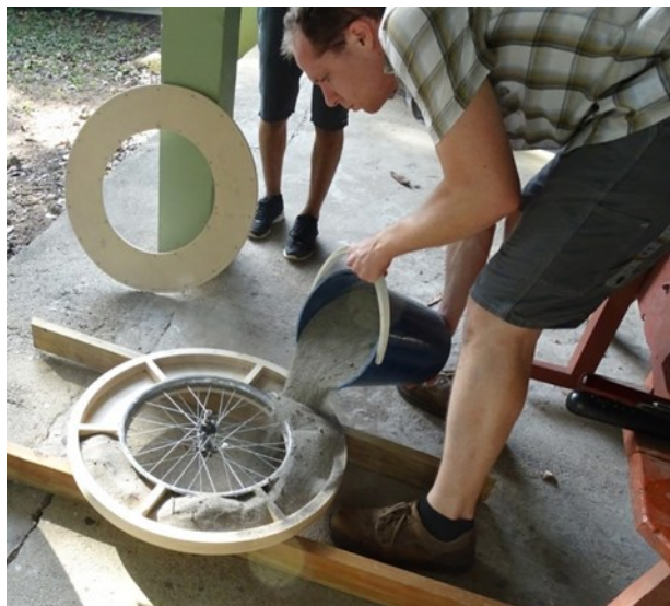
Filling the flywheel with sand to increase its momentum
