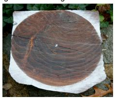
Additionally, I also use the spray paint for marking the extent of the center of a log that needs to be chainsawed out to remove enough of the pith so the half rounds will hopefully not start getting pith cracks right away. I used a folded newspaper as a mask, as well as to keep the paint off the patio. This is very helpful on any wood (such as this cherry), but particularly on dark woods like walnut where other types of marks are not very visible.
