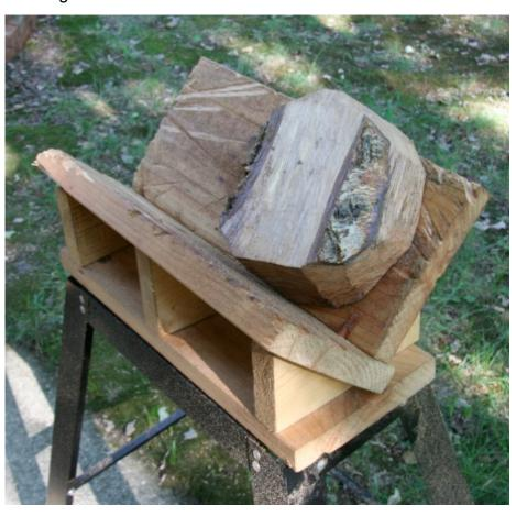
Because everything near the saw is wood, the chain can never come near metal – that's important. There are obviously many improvements that could be made. The V boards can slide around a bit now, and might be pinned for further constraint, but I haven't felt the need to make the effort. When I upgrade this one, I'll use larger dowels for holding the top V board in place – a really heavy log could shear the small ones I used in mod 1.
