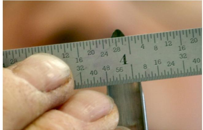
The cutting bevel is ground at about 40 degrees, but the heel is relieved to a smaller angle to make it fit into small places.
