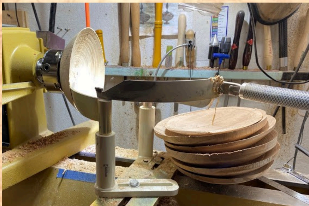
Jeff Struewing - first turned a bowl form and now in-process shot of coring very shallow with the Oneway Core Saver
