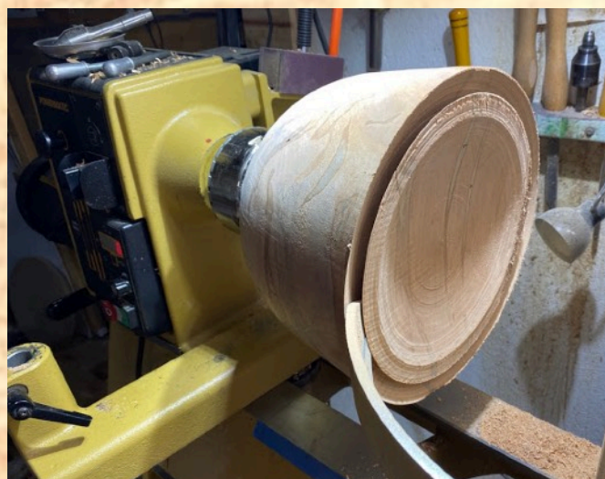
Jeff Struewing - first turned a bowl form and now in-process shot of coring very shallow with the Oneway Core Saver
