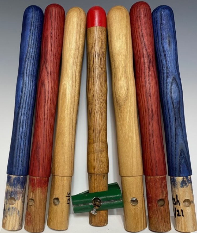
Jeff Struewing Saw Handles - 13" x 1.25" White oak (red), Ash (blue), Locust (natural)
