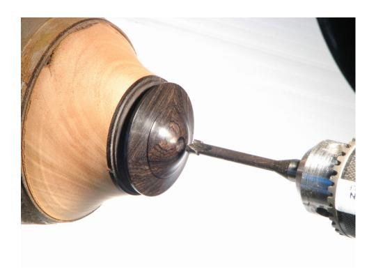
Here's the turned and finished base. I've also drilled a ¼" hole to accept the finial. Below is another shot. The diameter should be cut to size as well.
