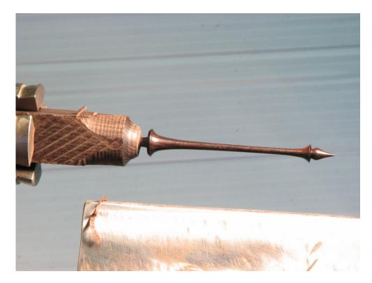
Here is the turned and finished top section. Notice the tenon to be inserted into the accent wood. Blelow is the sections glued together (CA glue) and aligned with the live center. This is an easy way for me to get good alignment.
