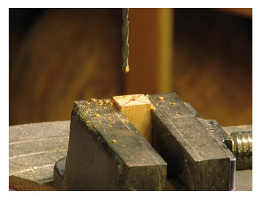
Drill a 1/8" hole in the accent piece of wood. Not all the way thru –just enough to accept the tenon. Again the surface should be flat to mate up to the bottom finial section perfectly.
