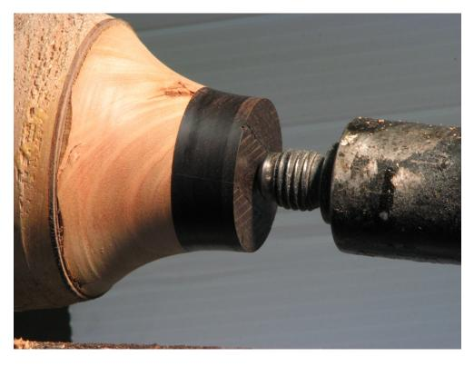
Turn the base round and just slightly larger than your finished diameter. Here, I've cut the waste block back in a nice sweeping arch-just because it felt so good to keep the cut going.
