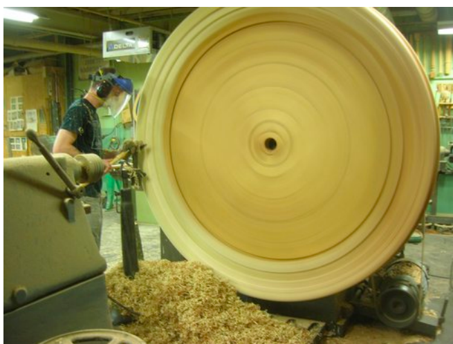
1943 Oliver Face Plate lathe. 40" diameter capacity.
