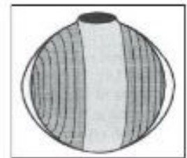
FIGURE 17 If this form is turned thin enough, the shrinking growth rings will force the pith outward into a football shape, instead of cracking.
