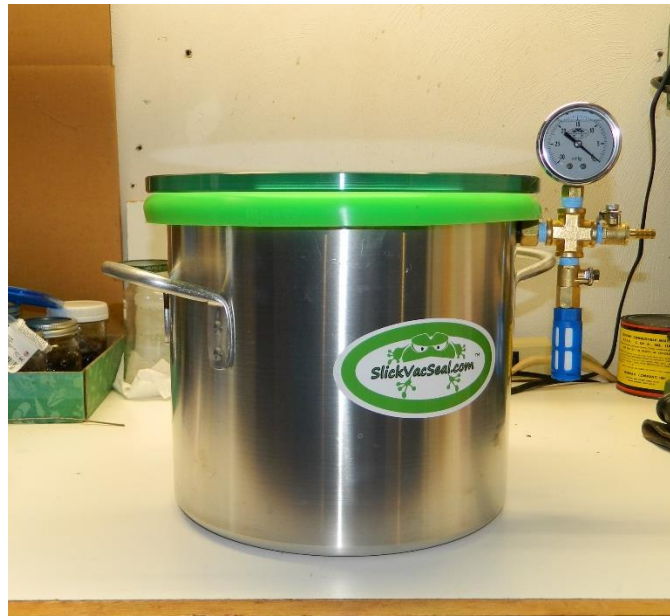
Figure 2 Three- gallon vacuum chamber, gauge, valves and filter
