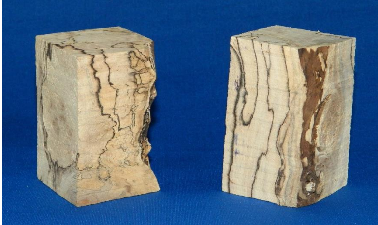
Figure 3 Pre-stabilization-process, dried, spalted-maple bottle stopper blanks. Size 1.5" square x 2.25" long.
